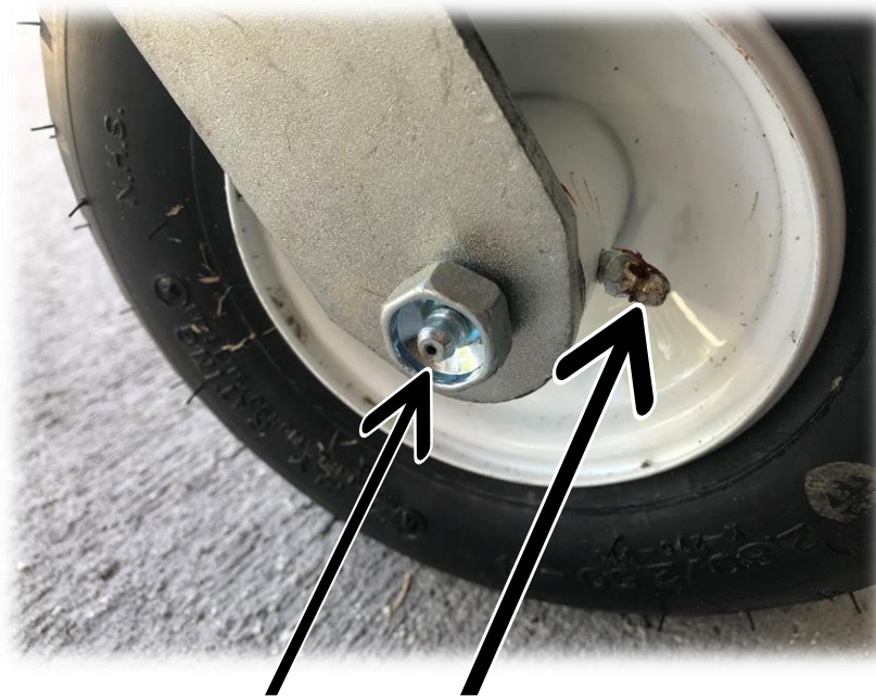
Location of rear axle bearings (Grease at either location)
